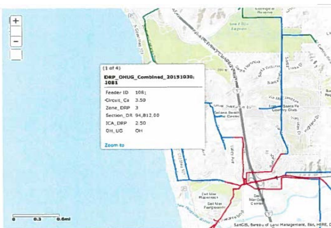
Figure 3 - Portion of SDG&E service territory, from publicly-available DRP map. 31 Red lines, Zone 1 of feeders (most proximal to substation); blue and green lines, Zones 2 and 3 of feeders. Substation is located northwest of Del Mar Golf Center in southern area of map, immediately west of Highway I-5. Pop-up box from Zone 3 of feeder
